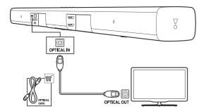
An Optical connection supports digital audio and is an alternative to an HDMI audio connection.
